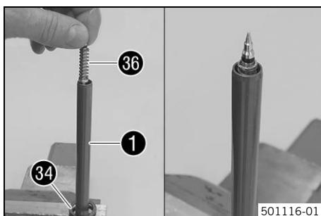
**Assembling the piston rod****Right fork leg**
