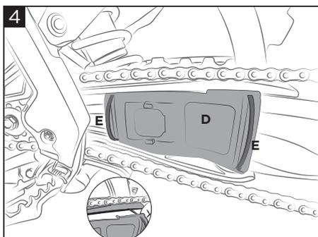
**Place the support (D) identifying the anchor points, insert the zip ties (E) as shown in figure and close them.**
