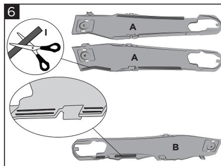
**Recommended application: Cut the adhesive rubber strip (I) using the length of the various ribs as a reference and apply it to them on both covers.**
