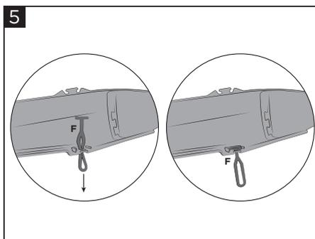
**Insert the rubber band (F) in the dedicated space, as shown in figure on both protections.**
