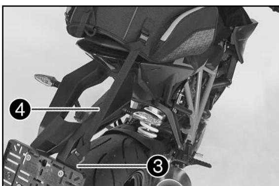
As an option, the fastening straps ④ may also be mounted on the license plate. To do so, mount the fixing loops ③ (included) using the upper license plate screws on the left and right, and then thread the fastening straps ④ through the loops.
