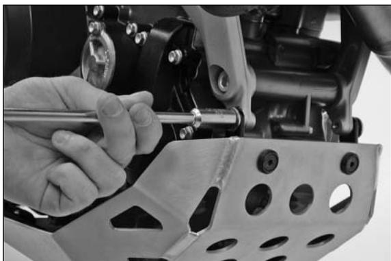
Tighten hex screws M6x16 of the front holding bracket to 15 Nm.
