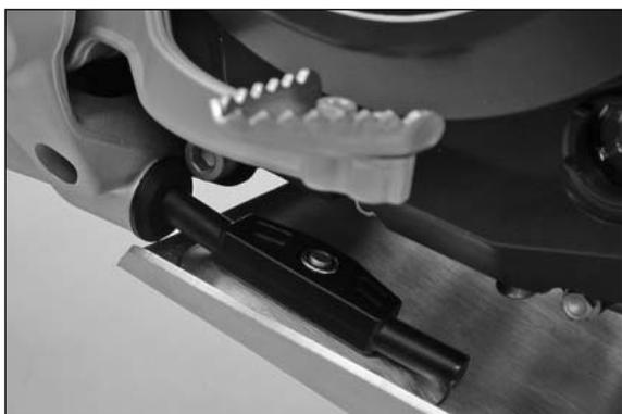
Insert the brackets of the aluminum engine guard into the rubber sleeves.
