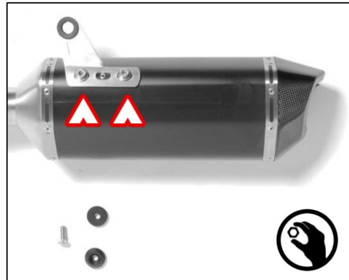
Mount both spacers onto the previously installed bracket.
